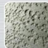
Another form of corrosion, which occasionally occurs in stainless steel sink bowls, is pitting of the surface; in extreme cases this may lead to perforation of the metal. The reason for this corrosive attack can usually be attributed to certain household products, for example:-
